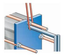
Straps should be used when lifting. Place straps according to picture.
