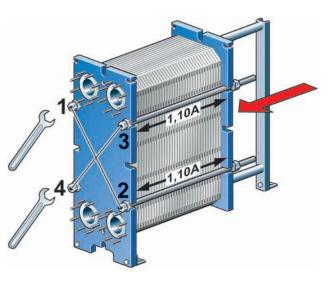
After that bolts are tightened alternately and diagonally, as shown in the figure below.
